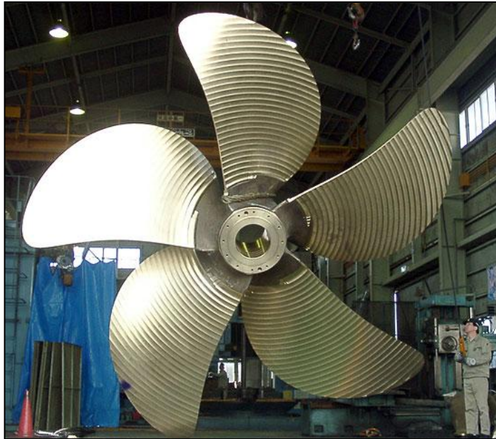
Abb. 3.2: Fixed Pitch Propeller (FPP) [KAMOME, 2010]
