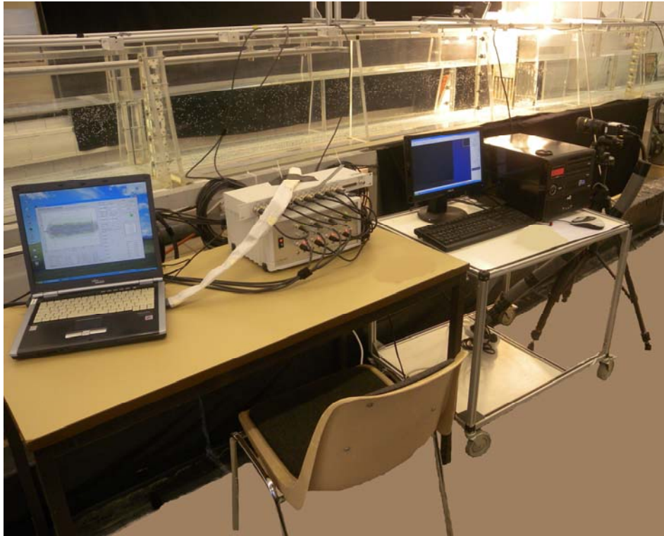
Photo 4.7: View of measuring devices for wave profile and wave velocity.
