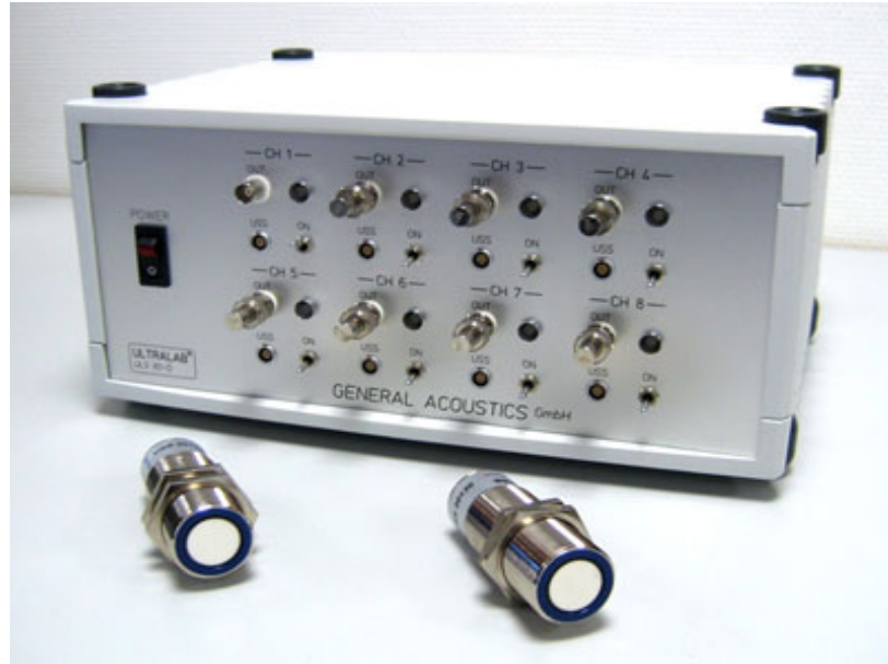
Photo 4.8: View of sensors and Ultralab. [87]
